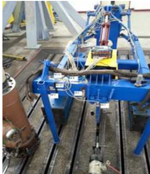
Fig. 2 - Locations of strain gauges M5, M6, M8, M9, M10, M11
