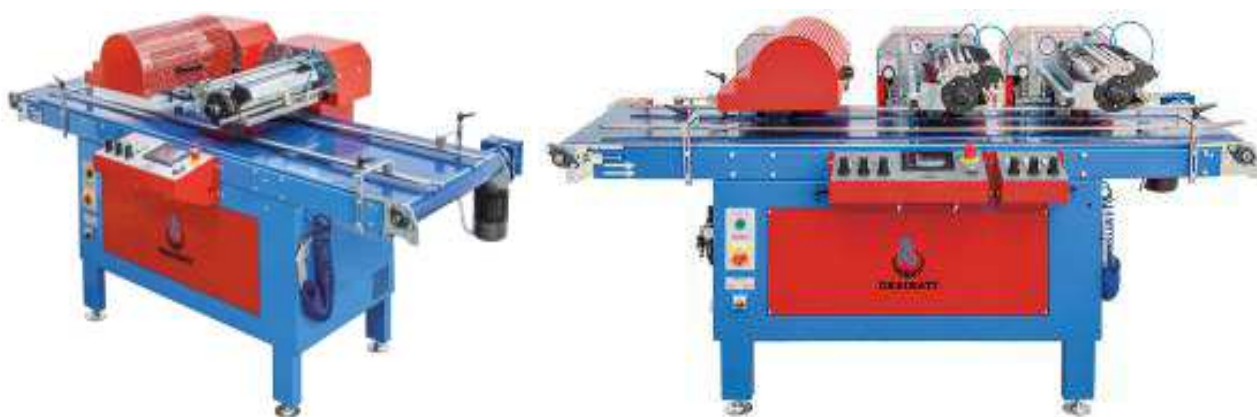
Fig.4 - LAMBDA drum seeder with one seeding unit and two from URBINATI. [18]
