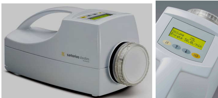
Fig. 1 – The portable air sampler SARTORIUS AirPort MD8 [5] (general view - left, control panel - right)
