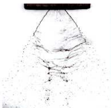
Fig. 5 - The way of dispersion of the liquid at the hydraulic spraying Source: documentary picture of the company LECHLER
