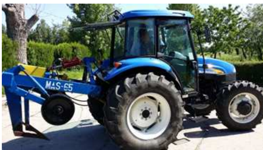
Fig. 1 - MAS-65 machine in aggregate with tractor New Holland TD80
