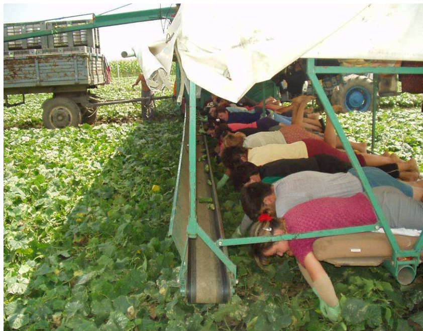
Fig. 1 - The mass transport on the belt conveyor and the position of picking personnel on the machine
