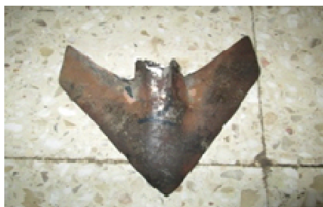
Fig. 7 - Breaking of the sweep blade
