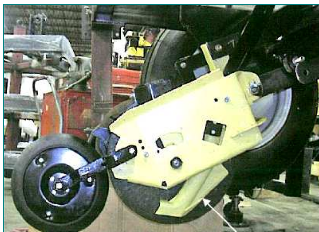
Fig. 4 - The Truax Rangeland Planter Boot installed on the planter
