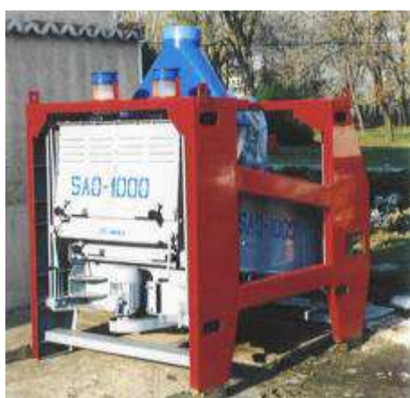
Fig. 1 - Separator vacuum swing - SAO 1000 (Overview)
