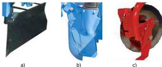
Fig. 4 -Types of plows of energetic willow planting equipment: a) plow anchor b) cultural plow, c) disc plow type [12], [13], [14]
