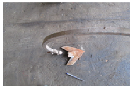
Fig. 8 - Broken sweep blade at the end of the experiment field
