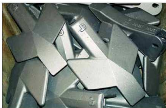
Fig. 6 - These John Deere Laser-Rip ripper points were produced in CADI for wear resistance and toughness in abrasive, rocky soil
