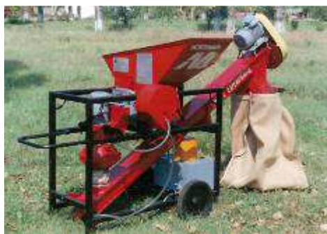
Fig. 1 - Seed treatment mobile installation with liquid solutions – IMTS 2 [5]
