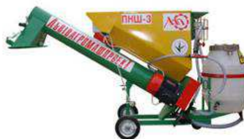
Fig. 2 – Seed treatment machine with screw conveyor with brushes, MTS-3 [6]
