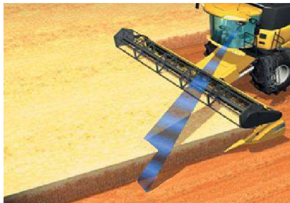
Fig. 4 – Alternative systems for combines autoguiding (with laser-left, with tracers-right) [www.newholland.com]
