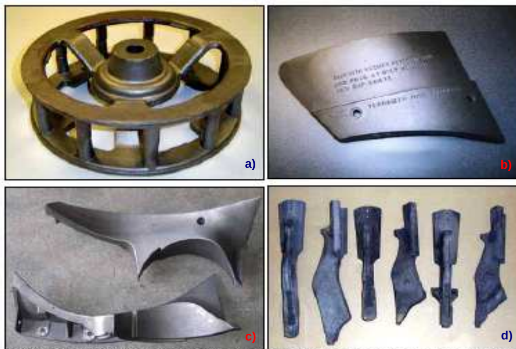
Fig. 2 - a) a one-piece ADI main drive wheel replaced an 84-piece steel welded and assembled component in the Toro Dingo TX; b) typical ADI plow point in production for more than 25 years; c) grain deflector for a harvesting combine is produced in ADI to stand up to abrasive grain flow; d) Australian farmers have utilized ADI Mitch Tips since the 1990s [4]
