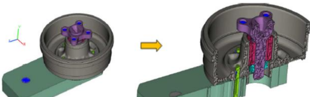
Fig. 3. Meshed model of the drum – steering knuckle plateau assembly / Modelul discretizat al ansamblului tambur – platou fuzeta
