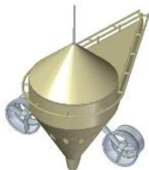
Fig. 5 – BM floating station for the monitoring of rivers' water quality / Statie flotabila BM de monitorizare a calitatii apei raurilor
