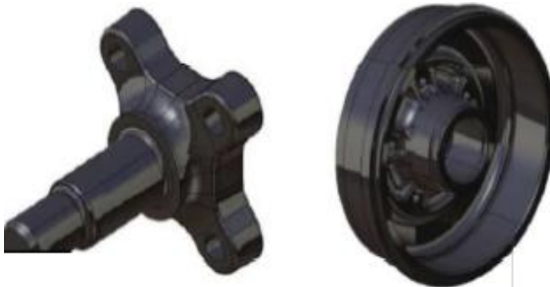
Fig. 1 – The 3D mode of the drum - steering knuckle plateau system / Modelul 3D al sistemului tambur – platou fuzeta
