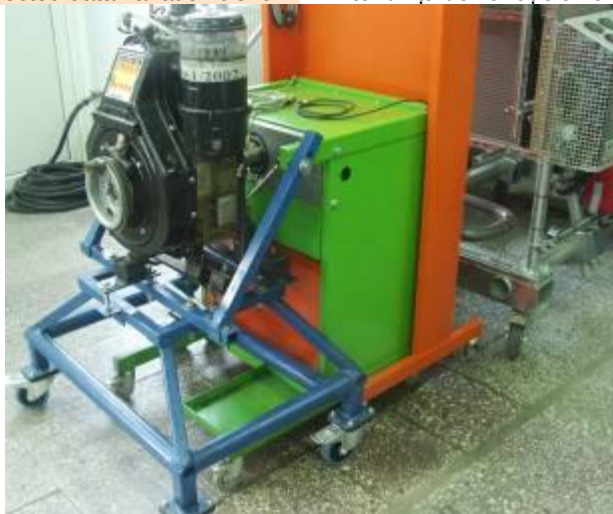
Fig. 9 - Single cylinder research engine test bed / Standul de testare cu motor monocilindric.
