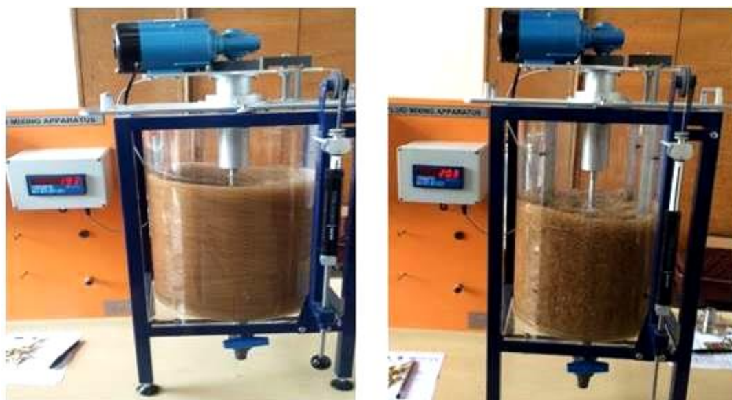
Fig. 4. – Mixing of Miscanthus x giganteus and water, without baffles (left) and with baffles (right)
