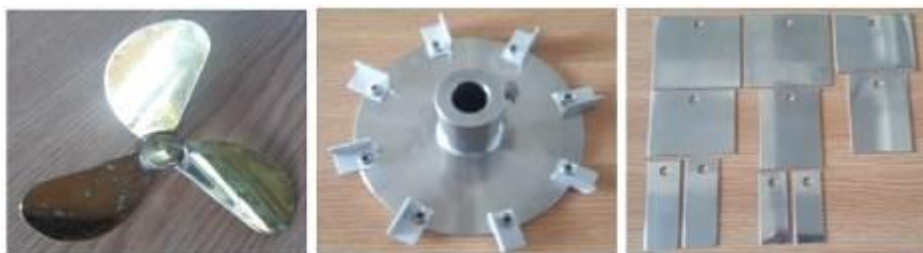
Fig. 2 - Types of stirrers used in the experiment: propeller, impeller turbine and blades
