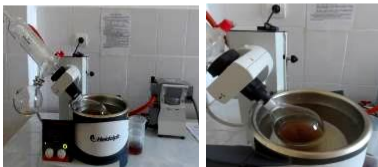
Fig. 6 – Rotary evaporator HEI- VAP BASIC 1 / G1B used for obtaining purslane extract concentrate
