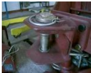
Fig. 17 – System of coupling tractor – trailer [6]
