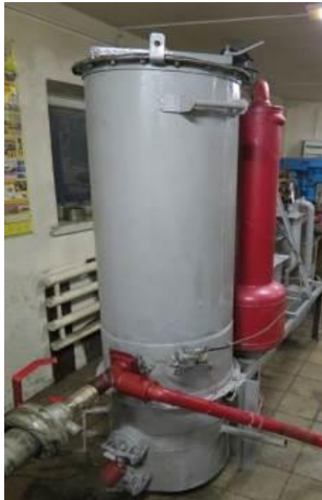
Fig.1 – Basic scheme (a) and general view (b) of the experimental installation where V_{gas} is gas producer productivity by gas, HCV_{gas} is higher calorific value of producer gas.
