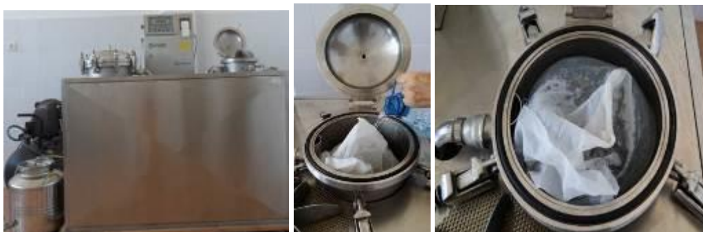
Fig. 5 – Timatic percolator by which means the purslane extract was obtained
