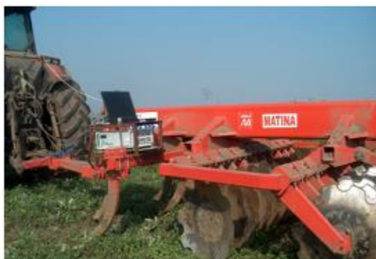
Fig. 18 – Aspect during the determination of traction force / Traction diagram of MATINA aggregate [5]
