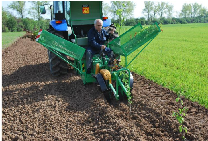
Fig.3 – MPF-1 Forestry sapling planting machine [3]
