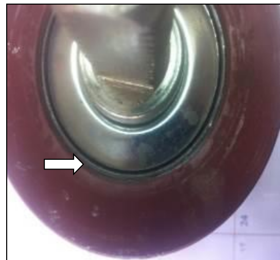
Fig.3 - The clearance between the roll rear cover and the roll.
