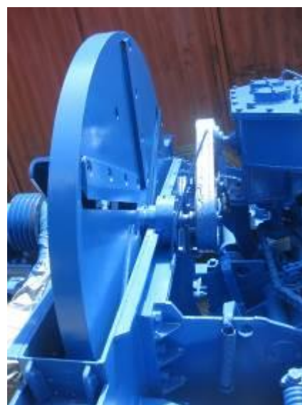
Fig. 4 – Chopping device with blades mounted on disk [12, 13]
