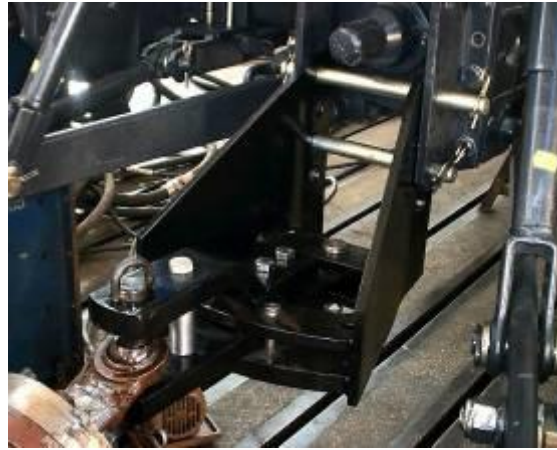
Fig. 27 - Fitting performed on Hydropulse installation for testing the swinging towing bar[11]
