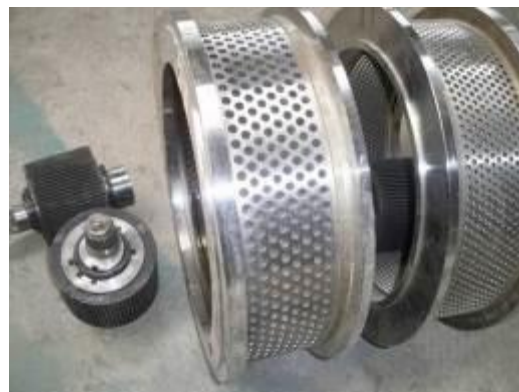
Fig. 3 – Examples of dies and pressing rolls (left – flat die, right – cylindrical die) [2, 15]
