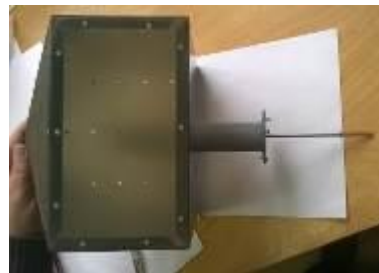
Fig. 9 – Assembling calibrated stem support in one of the models to measure air flow thrust force
