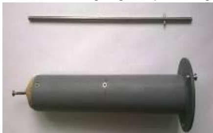
Fig. 8 – Construction of the support for calibrated stem used to measure thrust forces
