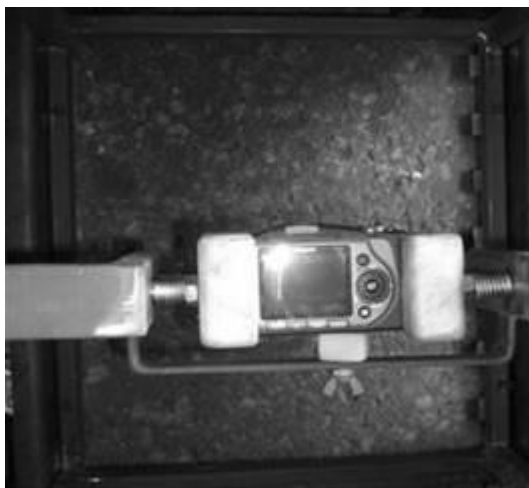
Fig. 3 - Digital camera mounted in sealed box on the autonomous robot
