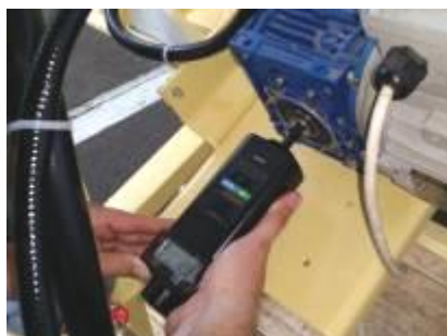
Fig. 3 - Aspect during revolution measurement output shaft of the gear motor, using electronic tachometer
