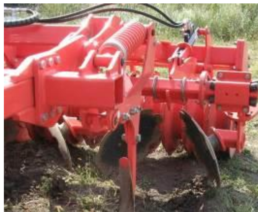
Fig. 3 - Battery of notched discs mounted in V shape, two by two (in the back)
