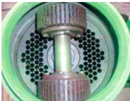
Fig. 3 – Examples of dies and pressing rolls (left – flat die, right – cylindrical die) [2, 15]
