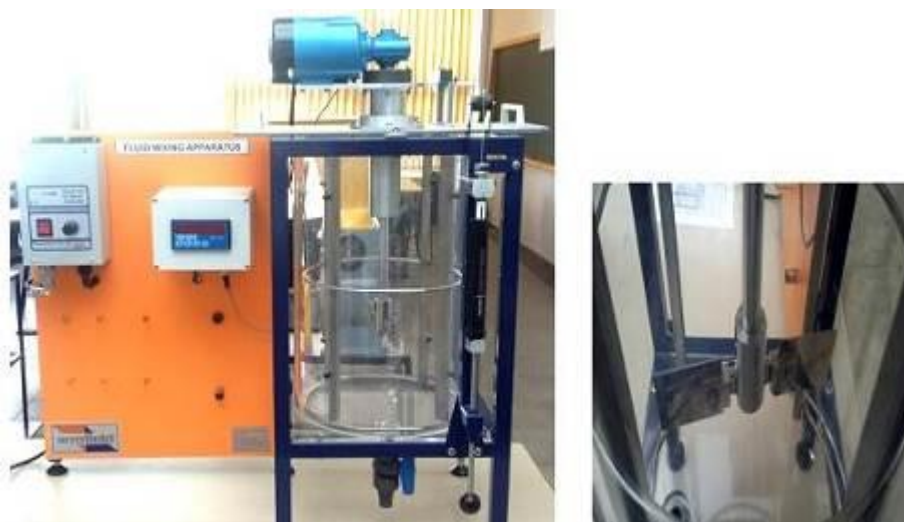
Fig. 1 – CEK Armfield stirrer for fluids, with the baffles mounted in the vessel
