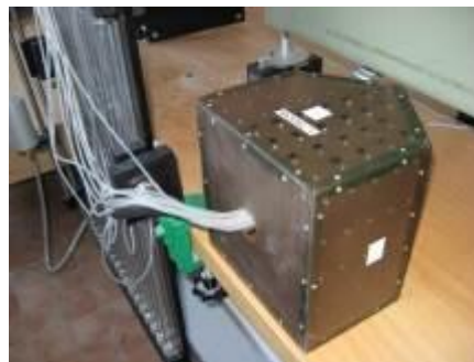
Fig. 5 – Preparing model 1 for measuring wind pressure
