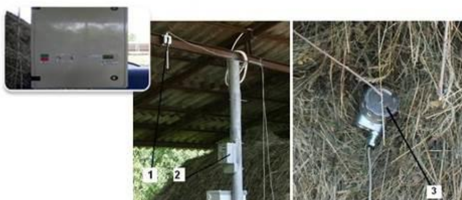
Fig. 3 – Command and control panel with temperature and humidity sensors location
