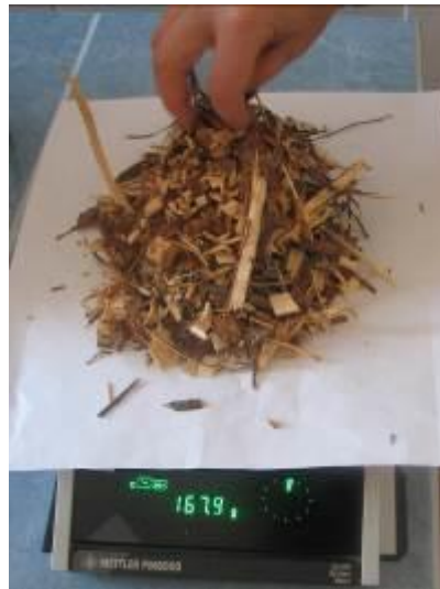
Fig. 10 – Weighing the chippings using Mettler PM 6000 device
