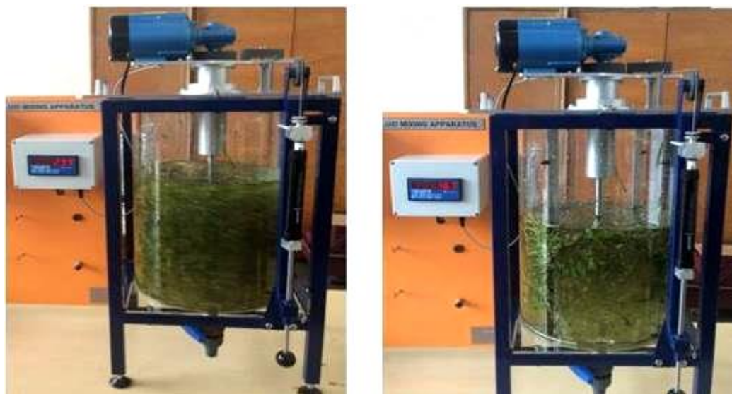
Fig. 5. –Mixing of grass and water, without baffles (left) and with baffles (right)
