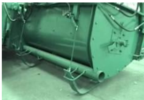
Fig. 3 - Probes mounted behind the header on the right. One can also notice the rod acting the rotary potentiometer, which conveys a signal about the position of the probe to the automation system
