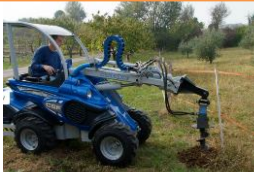
Fig.4 - GT series fitted with drilling equipment [8]
