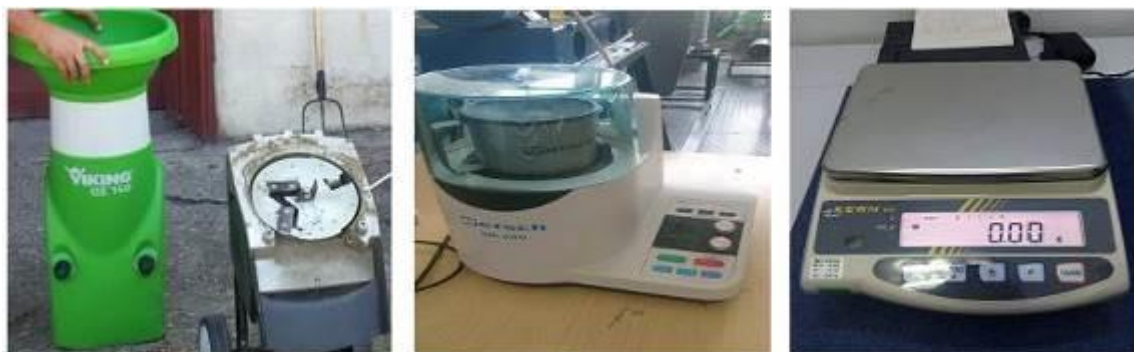
Fig. 3 - Viking GE 150 garden shredder, Grindomix GM 200 laboratory mill and Kern EW-N/EG-N balance used in the experiments
