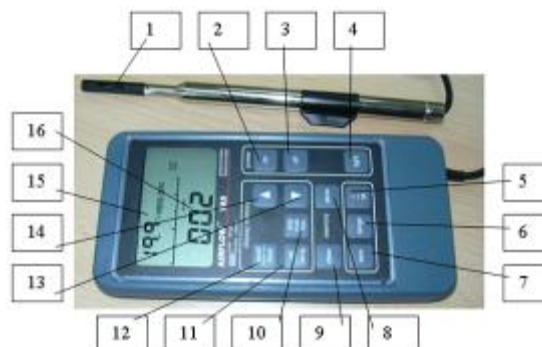
Fig. 4 – Thermal anemometer attached to the wing tunnel [13]
