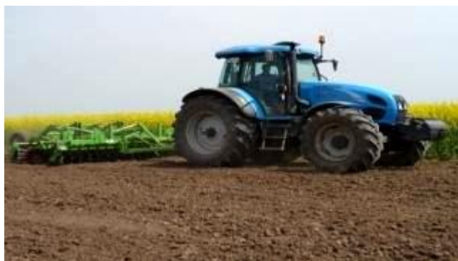
Fig. 12 - Aspect during working with GD-4 harrow with independent disk [4]
