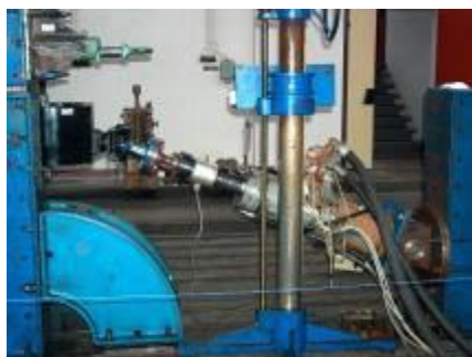
Fig. 23 - Fitting on Hydropulse installation for testing the assembly of device support – towing yoke [9]
