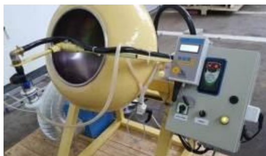
Fig. 4 Measurement of flow through the nozzle by using the nozzle tester
