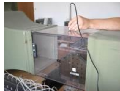
Fig. 7 - Model 1 fixed in the wind tunnel to measure pressures
