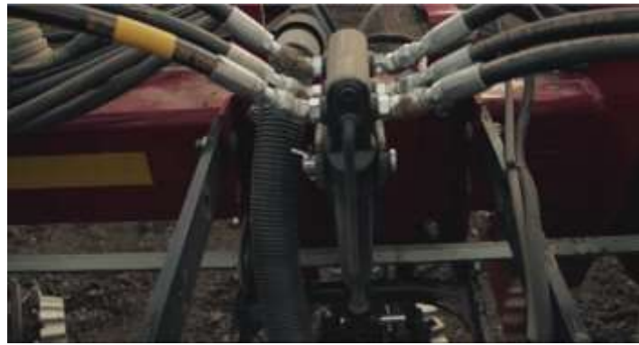
Fig.5 – Hydraulic drive for adjusting the seeding depth [11]
