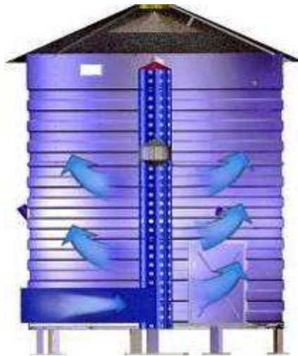
Fig. 3 - Aeration through a central column
