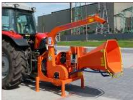
Fig. 16 – Forestry shredder Skorpion 280RB / 350 RB [8]
