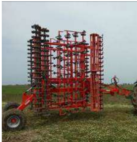
Fig.1 - Combinator with reversible-chisel and/or arrow type vibrating acting bodies used for conducting the experimental researches
