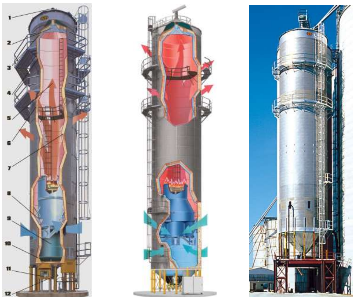
Fig.1 – Flow diagram of the GSI tower dryers [8]
