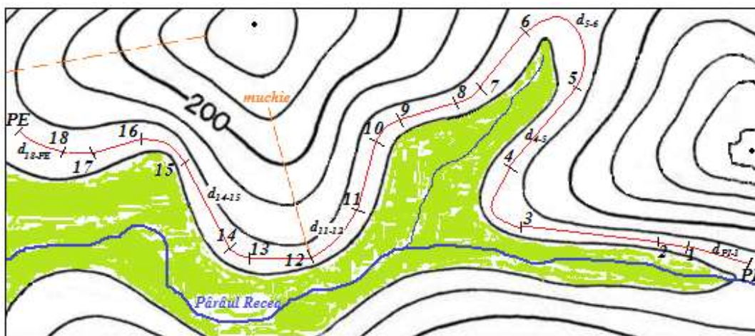
Fig. 2 - Scheme of location of a terrace placed between two level lines (level curve)
