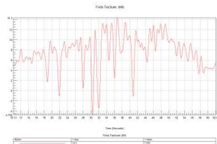
Fig. 7 - Variation in time of traction force for the aggregate made of technical equipment for establishing agro-forestry belts and wheeled tractor of 65 HP determined in experimental plot of C.C.D.P.C.P.N. Dăbuleni
