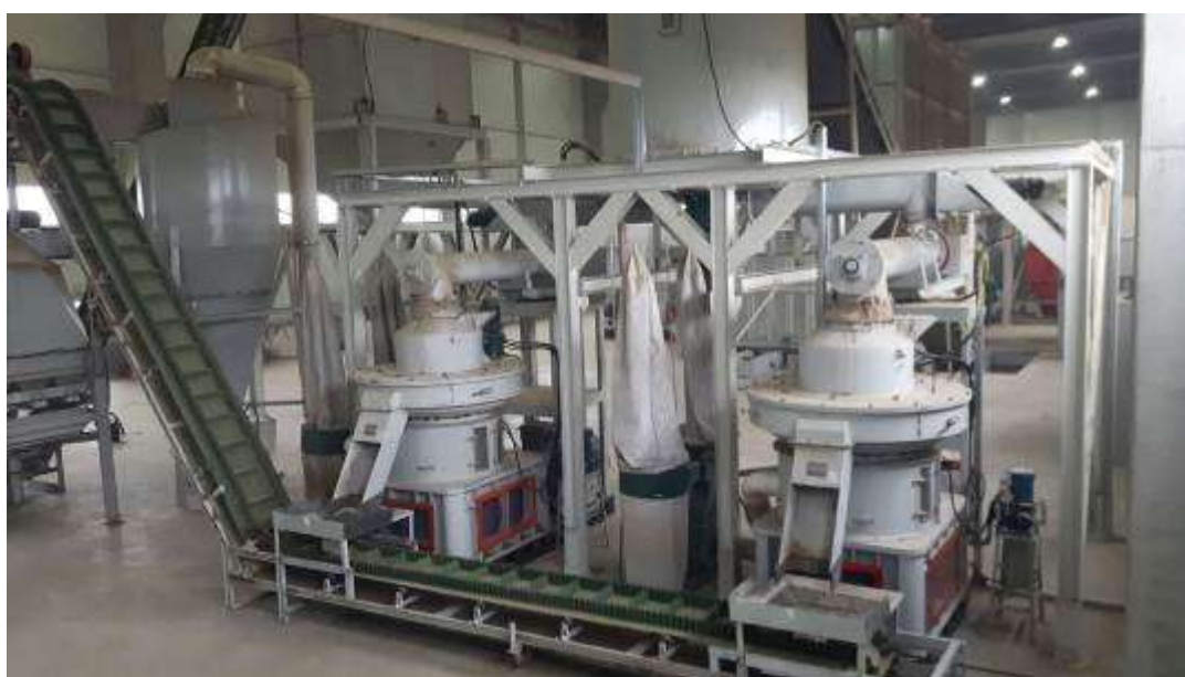
Fig. 1 – Ring die pelleting installation used for obtaining pellets
