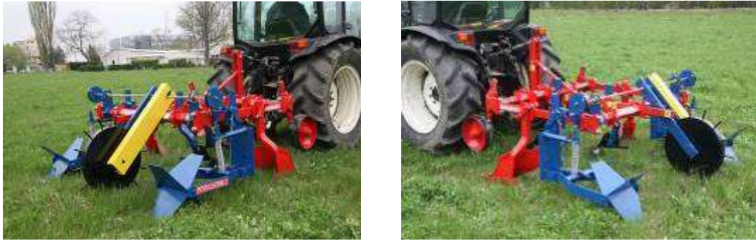
Fig 10 - Equipment for soil modelling in furrows compartmented on fruit and vineyard plantations. simultaneously in two furrows per interval. PCM2.2 + EMBC2-0 [6]
