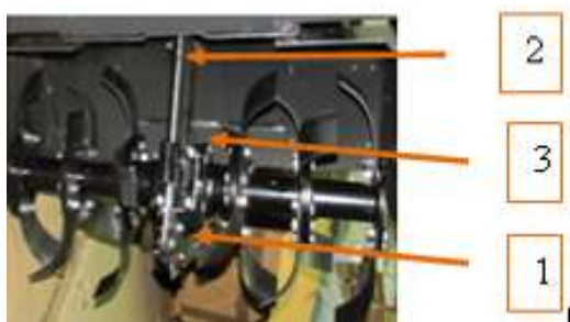
Fig.2. Adjusting the working depth 1 – mill coverage, 2- bolt; 3- performed rod
