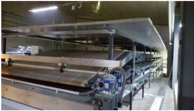
Fig. 5 - Tunnel prover with three conveyors (source: Pani Enterprise. Arges)
