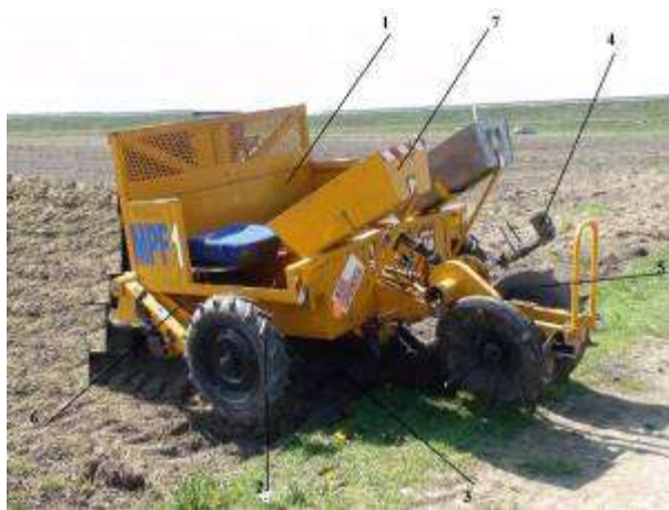
Fig. 12 - MPF1 seedlings planting machine [3.4]
