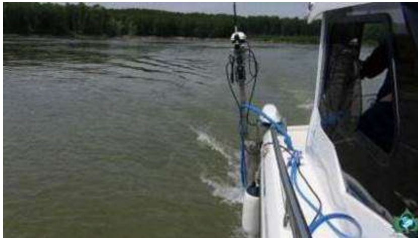
Fig. 5 - Kongsberg Geoswath Plus Compact System
