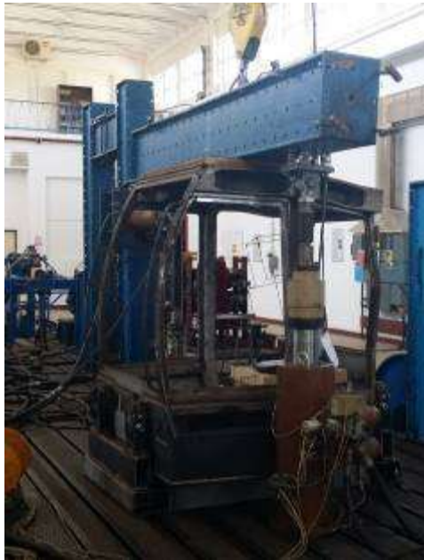
Fig. 4 - Montage realized on “HYDROPULSE” installation for HSM Hohenloher Heckscheibe - model 208F 20to cabin testing, in case of central crushing
