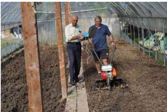
Fig. 5 - The system used for experimental measurement of hand-arm vibrations in the soil-processing activity
