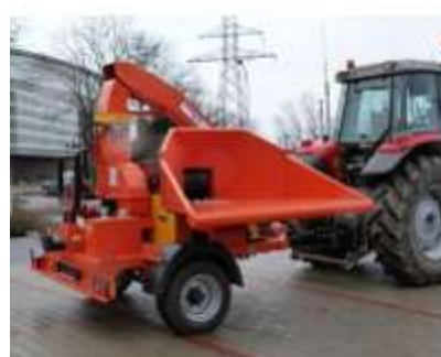
Fig. 16 – Forestry shredder Skorpion 280RB / 350 RB [8]
