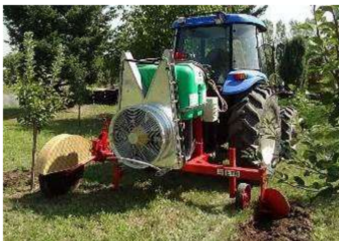
Fig. 1 – Technical equipment for soil work in fruit tree row concomitantly with the root cutting aiming a moderate growing of offshoots and the precision foliar fertilization
