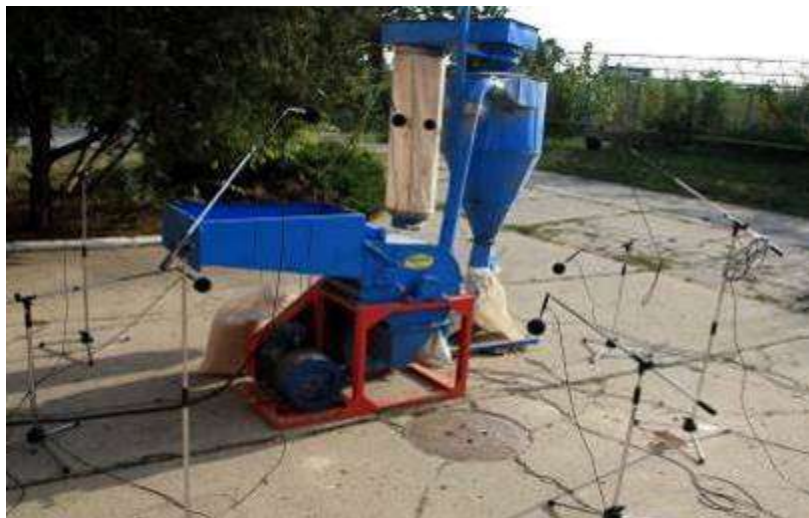
Fig. 5 – Determining the acoustic power level of the universal hammer mill (in the laden condition) by using Pulse system (9 microphones)
