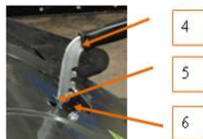
Fig.3 - Adjusting the shredding grade 4- handle, 5 – bolt, 6- compression spring
