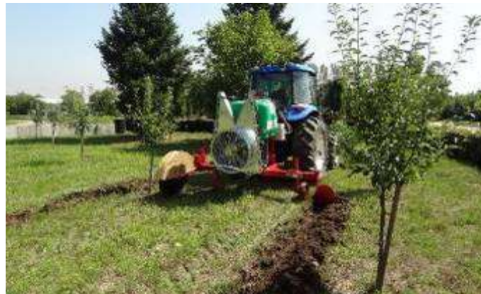
Fig. 5 - Aspect during the determination of energetic indexes for the aggregate TD 80D New Holland tractor + ETR technical equipment during root cutting and soil processing works
