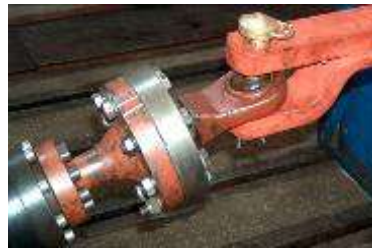
Fig. 3 - Installation on the Hydropulse plant for the static test of the draw bar
