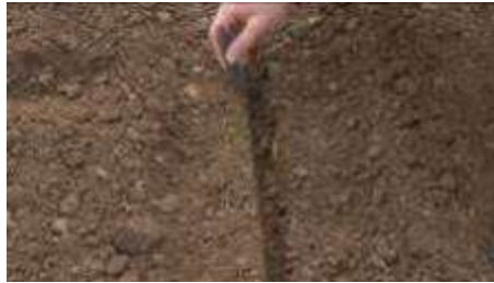
Fig.9 – Collapsed furrow sidewalls due to a force too small on the gauge wheels [14]
