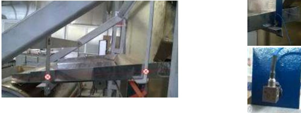
Fig. 4 - The accelerometer mounting onto the elastic elements
