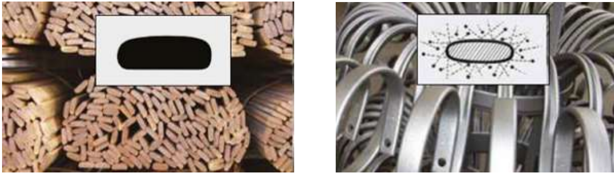
Fig.1 - Rolled convex steel used in the production of vibratory working tools
