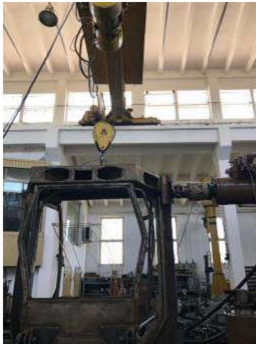
Fig.3 - Montage realized on "HYDROPULSE" installation for cabin testing in case of central crushing
