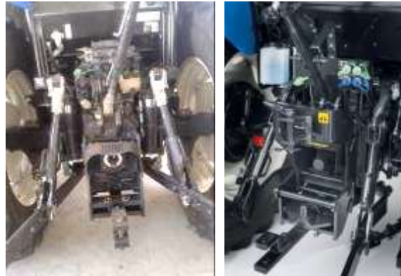
Fig. 1 - The coupling hook-type system of the lower coupling bolt
