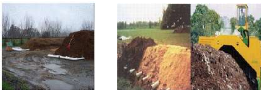
Fig. 2. Aerated static pile system with perforated pipes [8]
