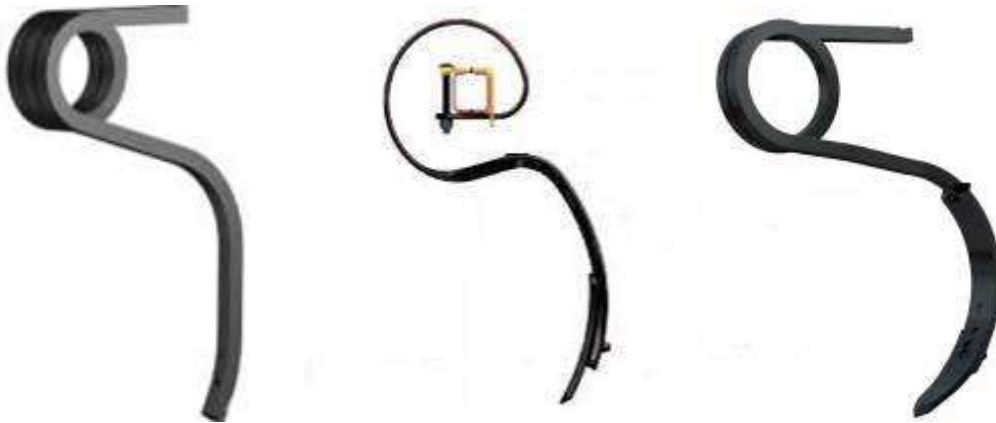
Fig.2 - Vibratory working bodies in which the spring is part of the working body shape [5]
