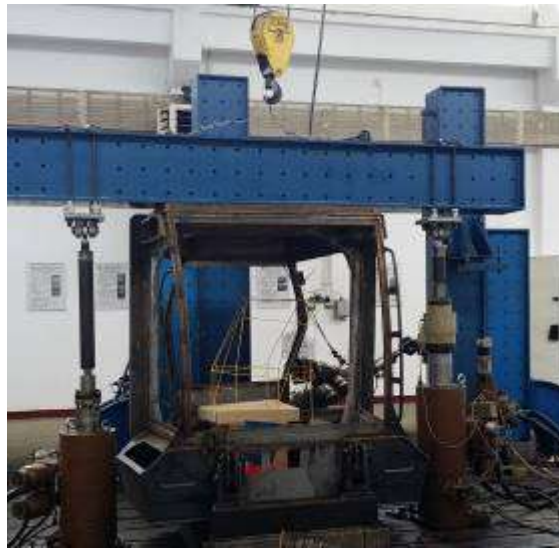
Fig.2 - Montage realized on "HYDROPULSE" installation for cabin testing in case of lateral load application
