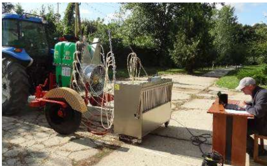
Fig. 4 - Aspect during the determination of uniformity of distribution of technical equipment on testing stand ED 20/900 E
