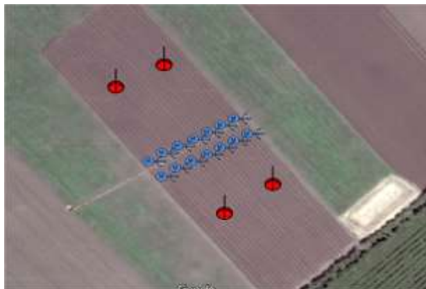
Fig. 9 - Emplacement map of the integrated sensors module and the valve control module for irrigation system on Tri Denal (Criuleni) farm
