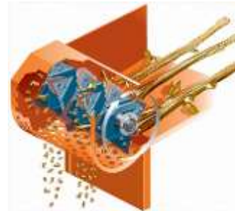
Fig. 20 – Shredder of branches ELIET SUPER PROF 2000 [9]
