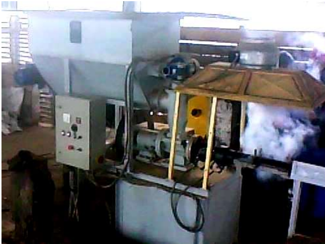
Fig. 8. Images of briquetting system of combined vegetal wastes
