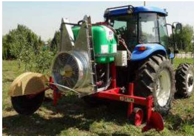
Fig. 1 - Technical equipment for working the soil in the row of fruit trees along with root cutting to moderate shoots growth and precision foliar fertilization, ETR
