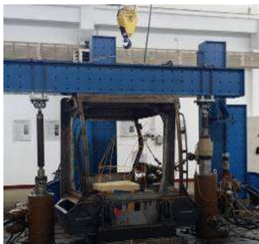
Fig.1 -Montage realized on "HYDROPULSE" installation for cabin testing, when the load is applied longitudinal.
