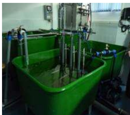
Fig.2 - Testing tank with water quality monitoring probes
