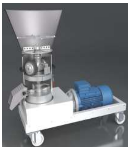
a-Flat die pelletization press and cylindrical rolls ;
