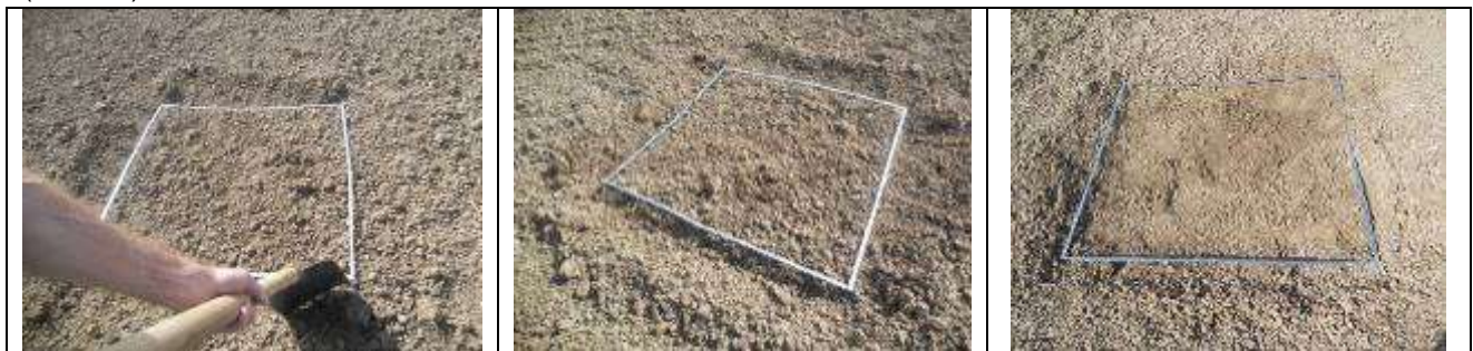
Fig. 6 - Aspects on how to determine the degree of soil shredding
