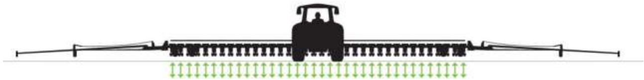
Fig.6 – Correct seeding depth maintenance on the entire working width using additional loading (pressing) systems fitted on each planting unit [13]
