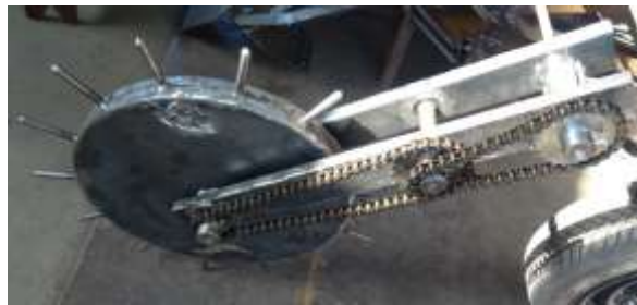
Fig.9 - Chain transmission for driving the rotor control mechanism [6]
