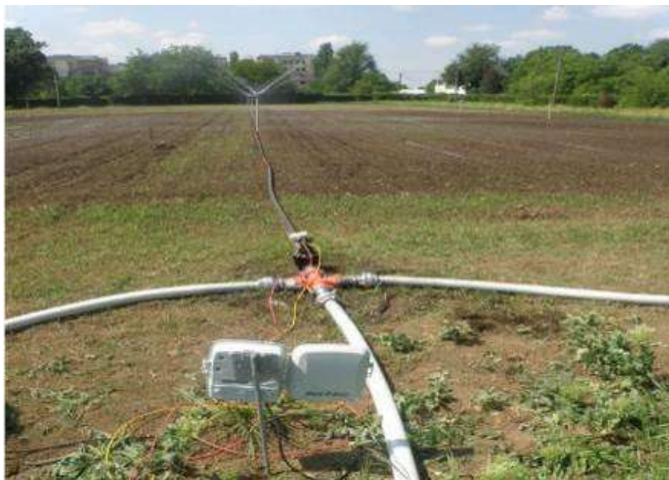
Fig. 9 - Sprinkle irrigation system wireless controlled
