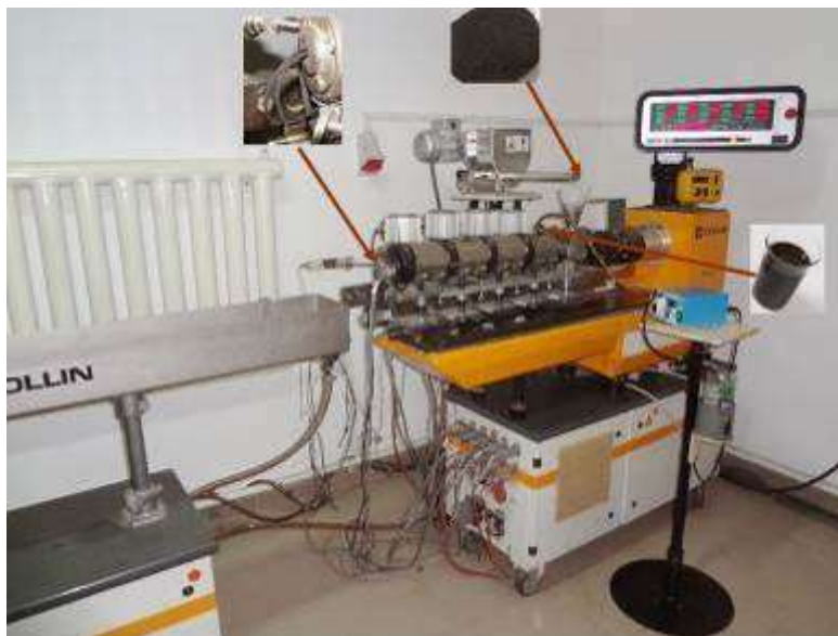
Fig. 2 – Extrusion plant type „ZK 25”, production Collin
