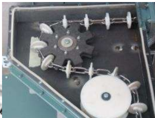
Fig. 13 - Manner of driving and changing the direction to return station with driving at TTL 90
