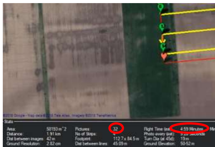
Fig. 8 – Display the number of pictures that the multi-spectral camera will take, as well as drone flying time
