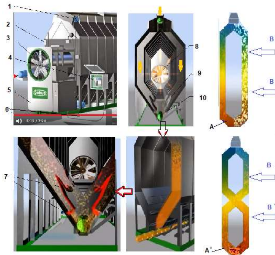
Fig. 7 - FSN cereal/seed dryer working principle and patent drying solutions [14]
