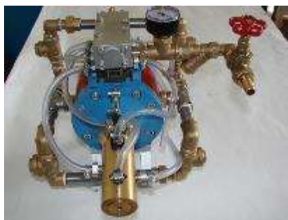
Fig. 9 a - Metering pump for injection of primary solutions - constructional version I
