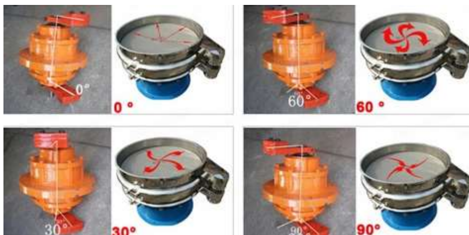
Fig. 16 - The vibratory- round sieves working parameters [18]
