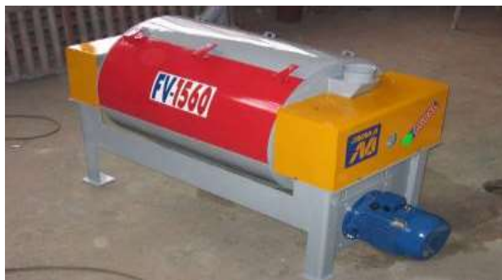
Fig. 1 – Vibratory finisher with self-cleaning
