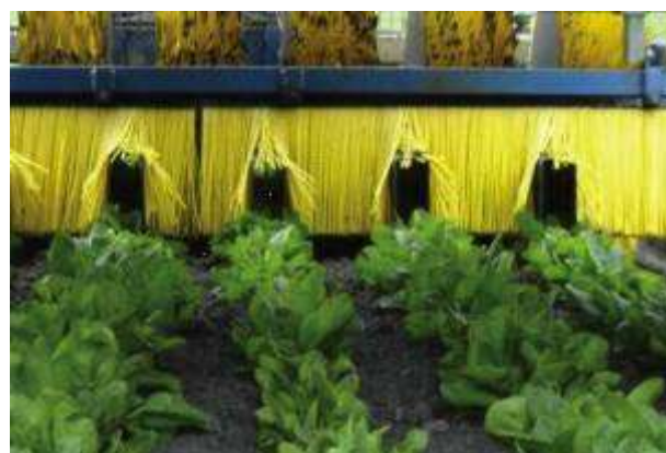
Fig. 8 –Fobro Hoe Brush tunnel cultivator detail (AGB)
