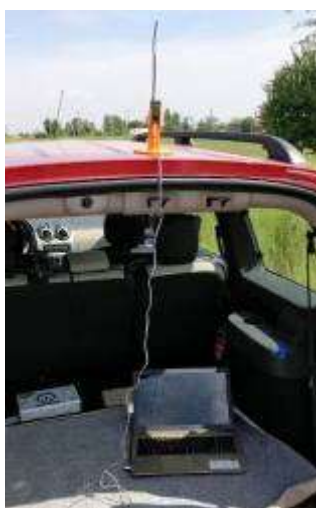
Fig. 3 – Telemetry antenna for monitoring flight parameters and the location on the map through the means of Mission Planner software
