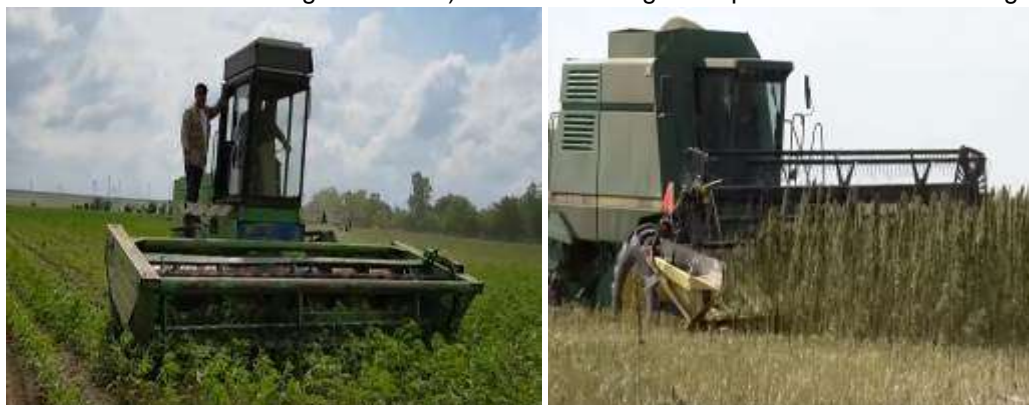
Fig. 10 - Shortening the hemp with windrower ( http://bhudeva.org )
