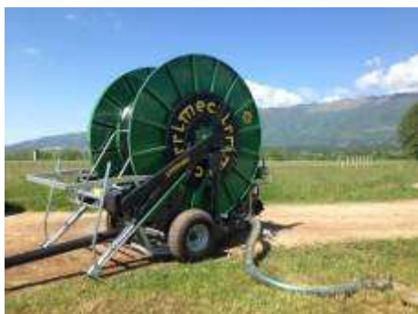
Fig. 8 - Reel drum irrigation system [14]
