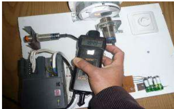
Fig. 8 - Measuring the speed of rotation of the metallic lamella with the electronic tachometer
