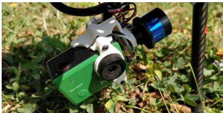
Fig. 4 – Multispectral camera gripping on the image stabilizer
