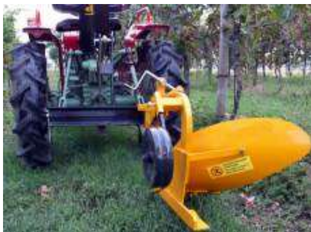
Fig. 6 - Plow with DP 18 model plow body for orchards marketed by Wirax
