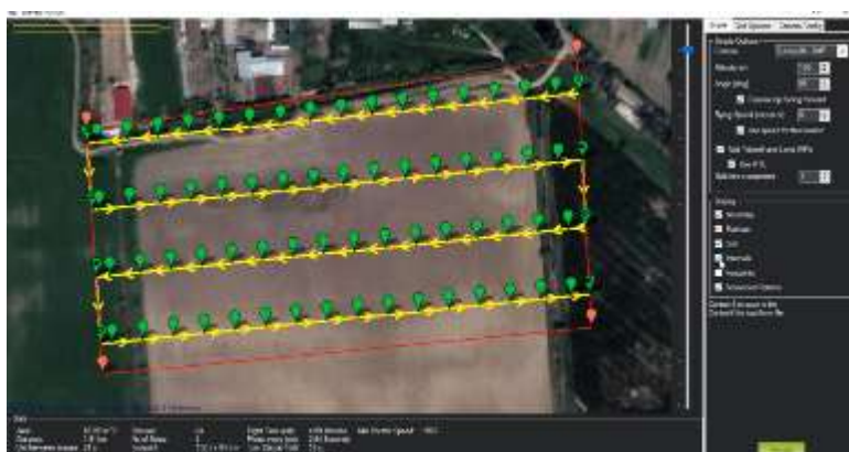
Fig. 9 – Displaying the points where the multispectral camera will take crop monitoring pictures
