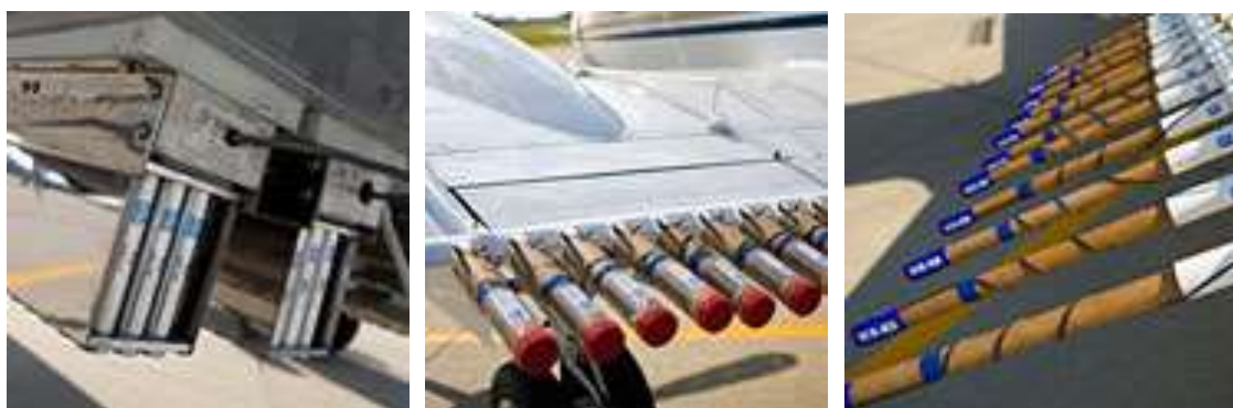
Fig. 12 - Pyrotechnic means used to combat hail by air [17]
