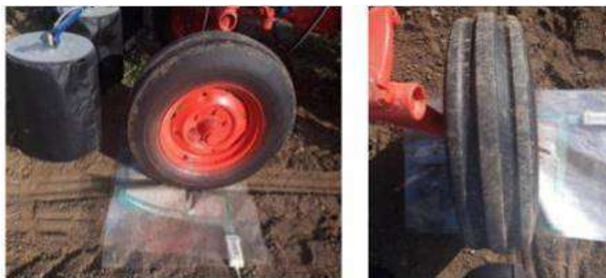
Fig. 4 - Front tire at minimum inflation pressure (100 kPa)
