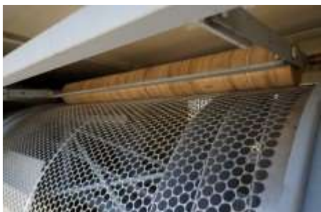
Fig. 6 - Rotary circular sievs and their cleaning systems
