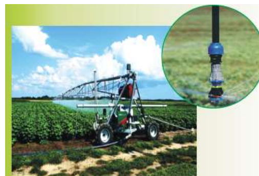
Fig. 9 - ramp and mobile pivot irrigation system [15]
