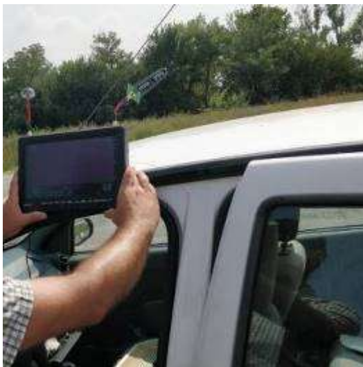
Fig. 10 – Live portable telemetry soil broadcast system
