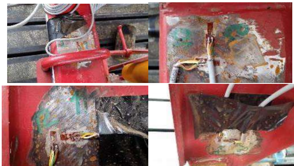
Fig. 2 – Applied strain gages on the frame - aspects
