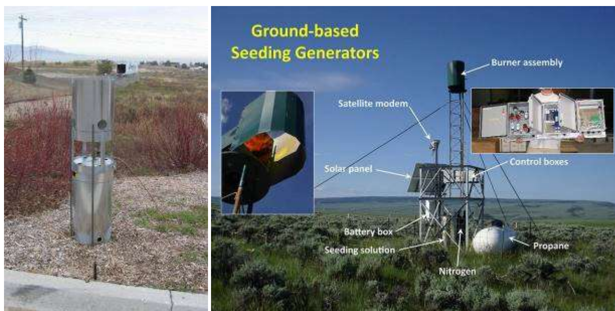
Fig. 13 – Ground-based generator (propane burner) [18,19]
