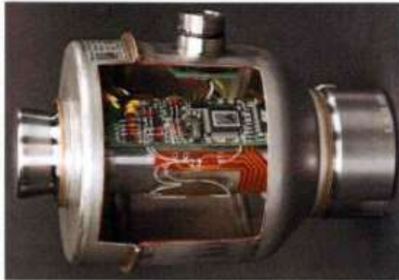
Fig. 3 - Section through a weighing cell with resistive transducer
