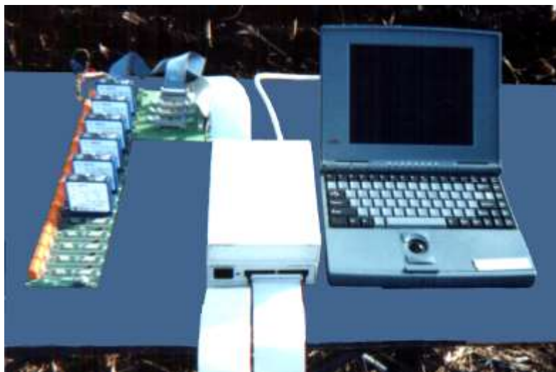
Fig. 6 - The system for measuring interaction forces tool-soil
