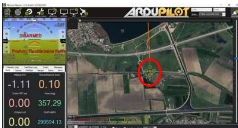
Fig. 4 – Setting the “Home” for the drone
