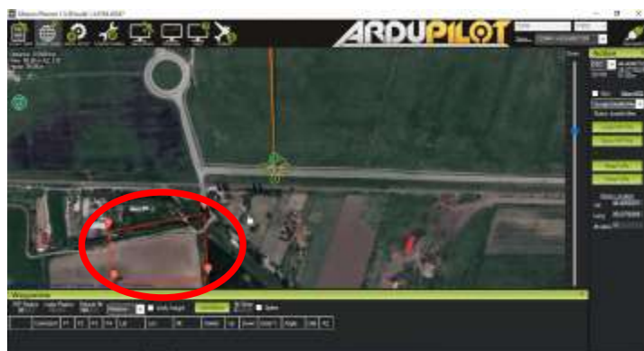
Fig. 5 – Setting the intermediate flight points
