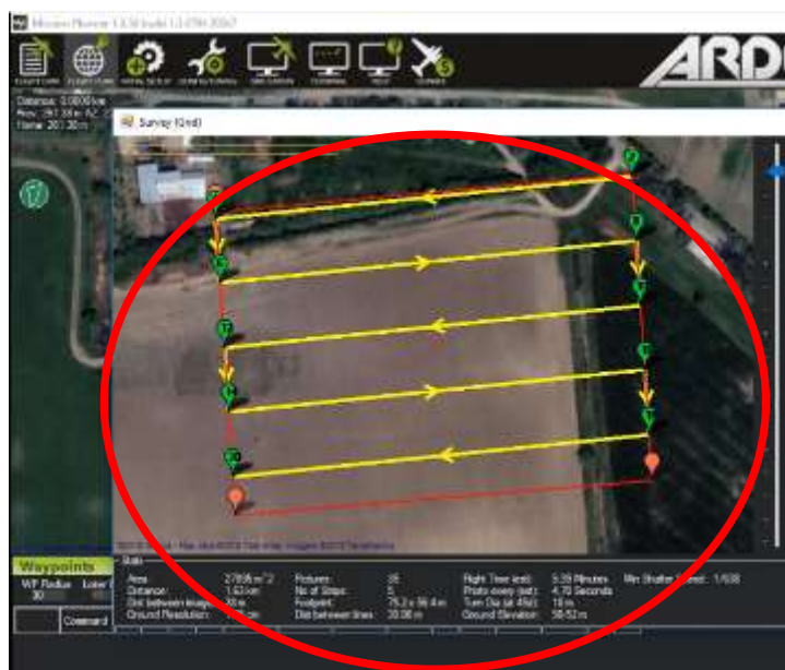
Fig. 7 – Generating the drone's flight path
