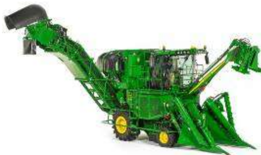
Fig. 1 – Self-propelled John Deere CH570 for harvester sweet sugar cane and sweet sorghum ( https://www.deere.com )
