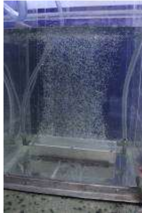
Fig. 11 - FBG with 152 orifices \varnothing 0.1mm in operation
