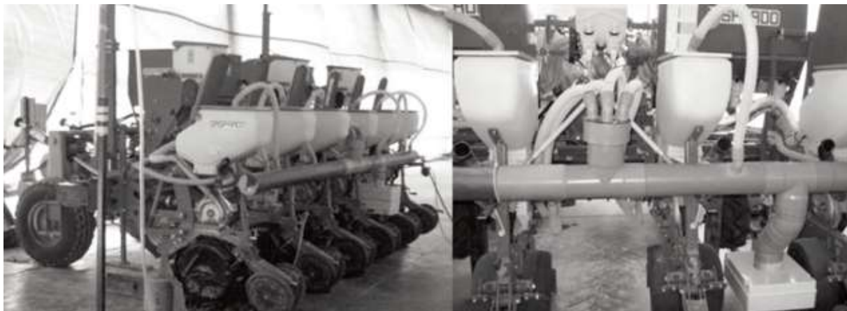
Fig.1 - The Gaspardo drill equipped with innovative systems developed at CRA-ING
