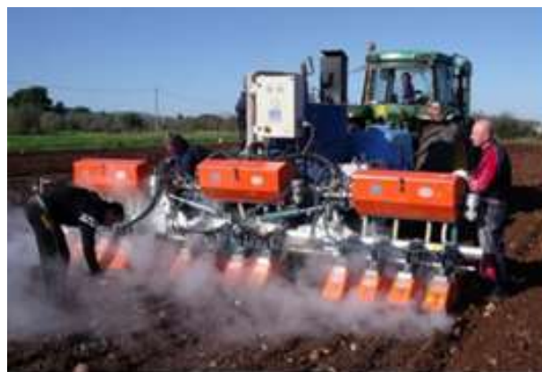
Fig. 4 – Machine for soil disinfection in strips (prototype) ( Raffaelli et al. 2016 )
