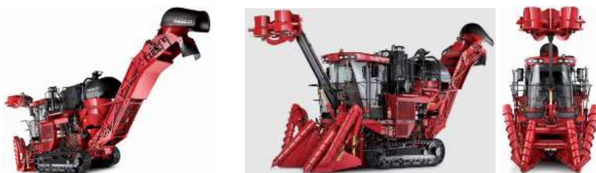
Fig. 4 – Self-propelled CaseIH A8000 for harvesting of sweet sugar cane and sweet sorghum ( https://www.caseih.com )
