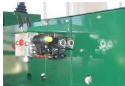
Fig. 4. b - Distributor drive cutting mechanism
