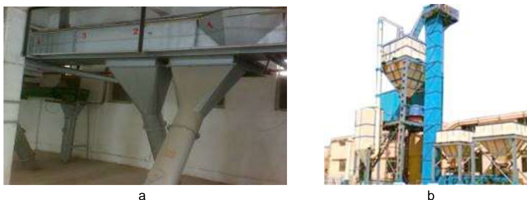
Fig. 2 - Conveyor belts system from a compound feed factory consisting of horizontal conveyor belts (a) and vertical elevators (b)
