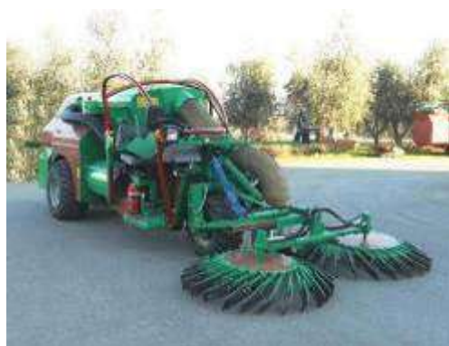
Fig. 3 - General view of self-propelled type pneumatic nuts collection machines
