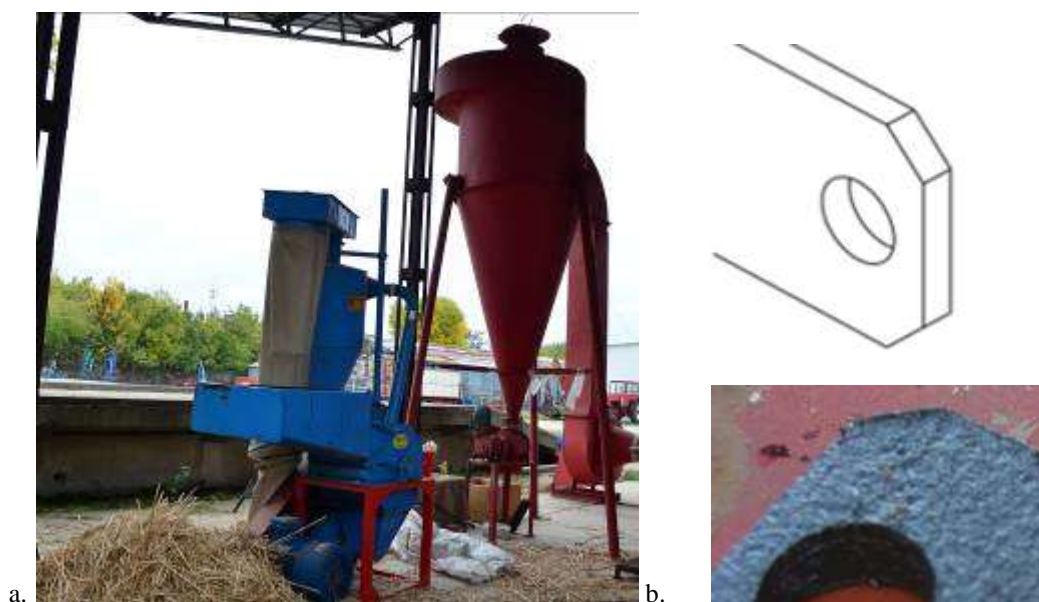
Fig. 1 – a. Hammer mill MC 22; b. Triangle edge hammer used for testing
