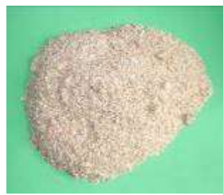
Fig. 7 – Refuse product on sieve with mesh of 630 µm
