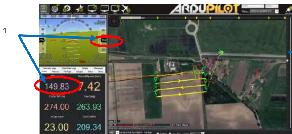
Fig. 11 – The actual start of the monitoring mission for the researched crop 1 – altitude set for the flight
