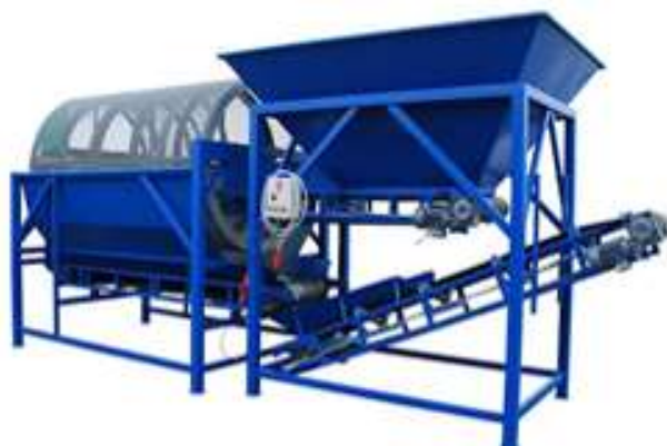
Fig. 7 - OPTION rotary sieve installation for separating grape seed from marc, Italy [9]
