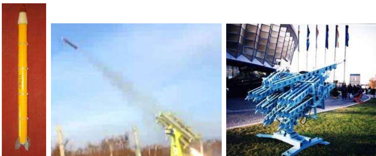
Fig. 9 – Anti-hail rocket RAG-96 and rocket launcher [10,14]
