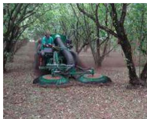
Fig. 3 - General view of self-propelled type pneumatic nuts collection machines
