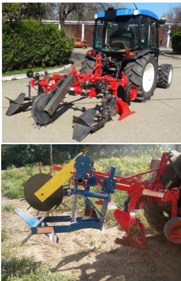
Fig. 3 - Equipment for soil modelling in compartmented furrows in vine and tree plantations, simultaneously in two furrows in the same space, PCVM2,2+EMBC2-0
